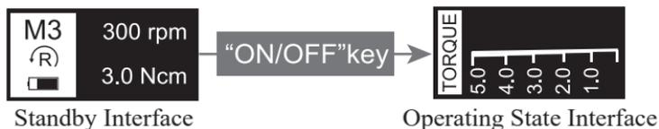
c) Standby interface and operating state interface of Reciprocating Motion Mode
