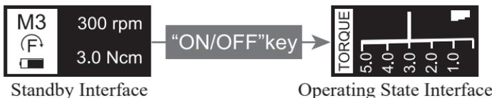
b) Standby interface and operating state interface of Reverse Rotation Mode
